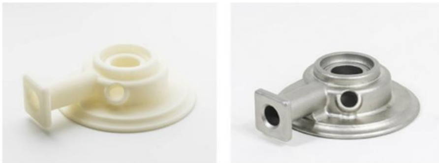
Figure 2.17 – An FFF printed pattern (left) and the final metal investment cast part (right)
