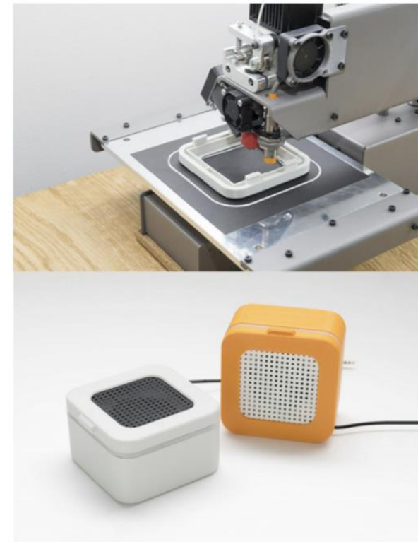
Figure 2.18 – The lid of a speaker enclosure being printed on a desktop FFF printer with snap-fit joints (top). The final assembled speakers printed from PLA (bottom)
