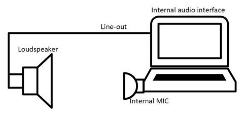
Figure 2 - Setup with an internal audio interface.
