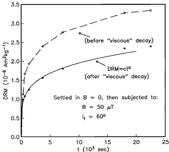
**Figure 9.** Magnetization versus time for redeposited recent river sediments. Dilute slurry settled in zero field, and was then exposed to a field for time  $t$ . Dashed curve is data measured immediately after exposure, and solid line is data measured after the sediment sat in zero field for a time equivalent to the exposure time. Parameters  $c$  and  $a$  were fitted as  $2.7 \times 10^{-7}$  and 0.211, respectively. Data from *Tauxe and Kent* [1984, also unpublished data, 1984].
