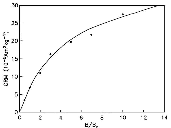
**Figure 6.** Plot of DRM versus applied field  $B$  for redeposited glacial varves.  $B_0$  is the field at the site. Dilute slurries were allowed to settle in an applied field, dried, and measured. Redrawn from *Johnson et al.* [1948].
