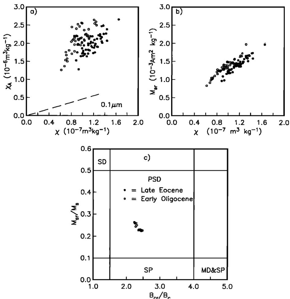
**Figure 16.** (a) Banerjee plot of data from marine carbonates from Site 522 (P. Hartl, unpublished data, 1992) and grain size predicted from *King et al.* [1983] (see Figure 14). Solid symbols are from the late Eocene and open symbols are early Oligocene. (b) Plot of  $M_{sr}$  versus  $\chi$  for same samples as in Figure 16a. (c) Day plot [Day et al., 1977] of hysteresis parameters for samples from two tracks shown in Figure 16b.
