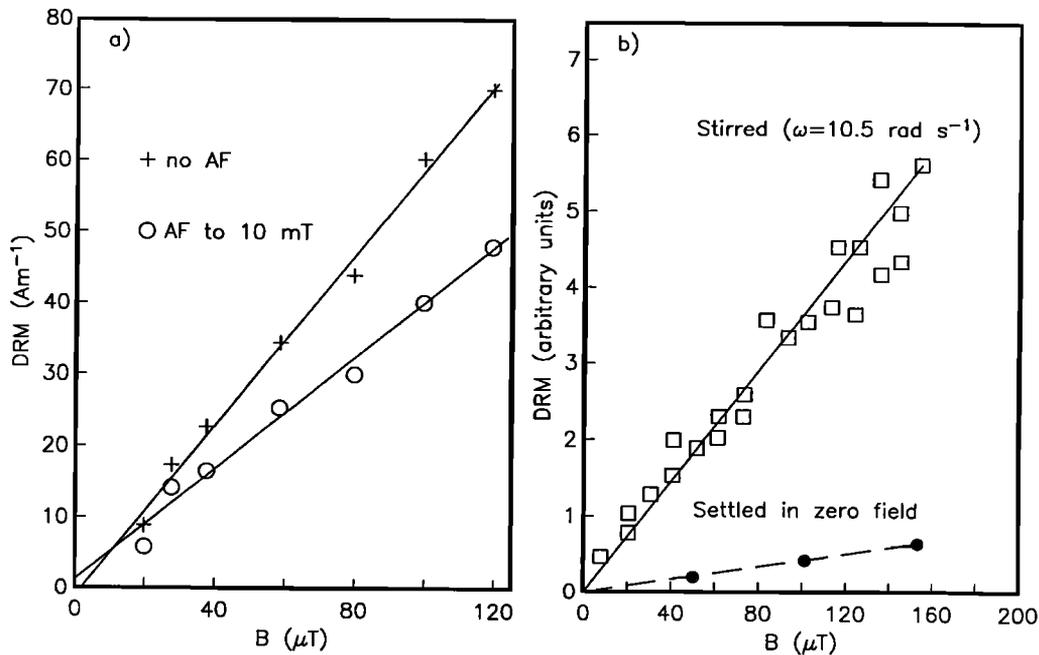
**Figure 11.** (a) Deep sea sediment redeposited in the laboratory. Thick slurry was stirred in the presence of field  $B$ . Redrawn from *Kent* [1973]. (b) Comparison of remanence acquired by stirring in an applied field (squares) versus that acquired when settled in zero field and then exposed to field  $B$  (solid circles). Redrawn from *Tucker* [1980b].
