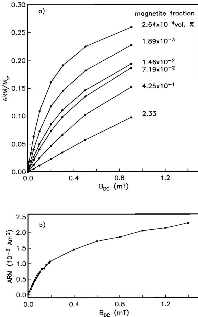
**Figure 15.** (a) Anhyseretic remanence normalized by saturation remanence versus the bias field applied during alternating field demagnetization  $B_{DC}$ . Redrawn from *Sugiura* [1979]. (b) Anhyseretic remanence versus  $B_{DC}$  for marine carbonates from the Ontong-Java Plateau.
