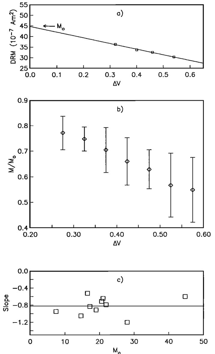
**Figure 12.** Data from *Anson and Kodama [1987]*. (a) Magnetization versus degree of compaction as represented by volume change ( $\Delta V$ ).  $M_0$  is the y intercept of a regression line through the measured data points (squares). (b) Same as Figure 12a, but all acicular data are normalized by  $M_0$  and averaged over 0.05-wide bins of  $\Delta V$ . (c) Slopes of all regression lines (see Figure 12a) versus  $M_0$ .
