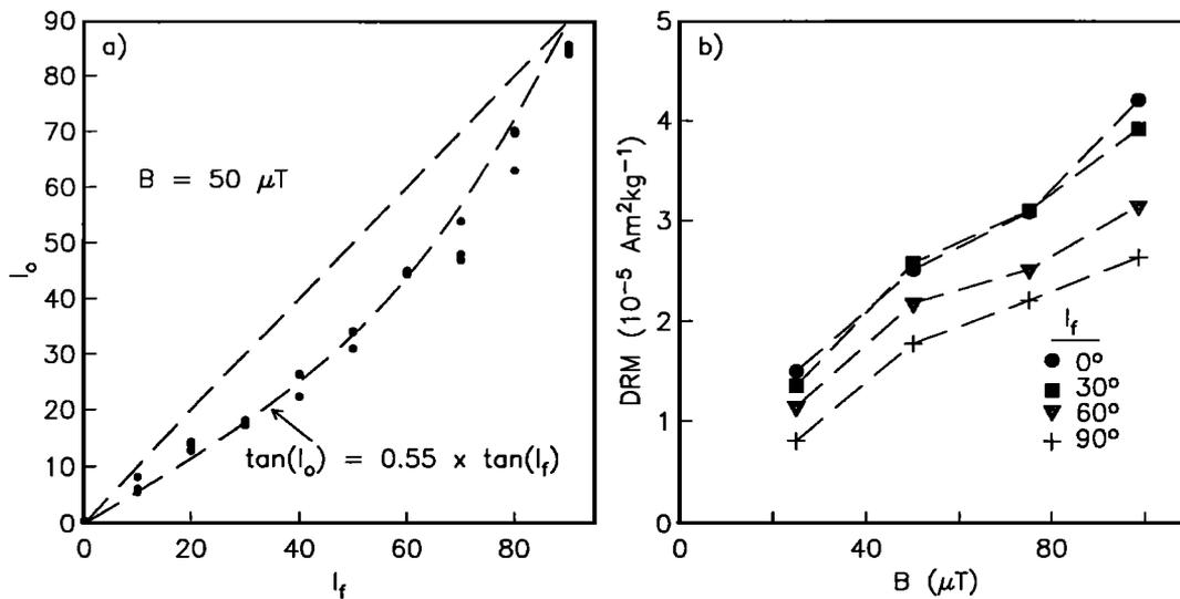
**Figure 7.** Data from redeposited recent river sediments, showing magnetization DRM versus applied field  $B$  for various inclinations. Dilute slurries were allowed to settle in an applied field; settling tubes were then inserted into a cryogenic magnetometer. (a) Observed inclination  $I_o$  versus inclination of the applied field ( $I_f$ ). (b) DRM versus  $B$ . Redrawn from Tauxe and Kent [1984].
