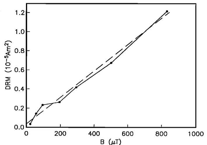
**Figure 8.** Magnetization versus applied field of redeposited lake sediments. Sediments were redeposited in a similar manner as those shown in Figure 7. Redrawn from Barton *et al.* [1980].
