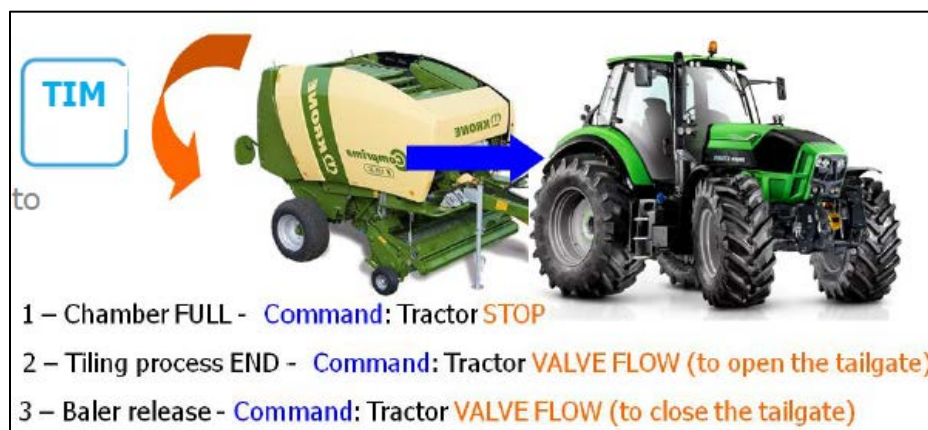
Figure 1. Commands from the implement to the tractor for a Krone baler (Source: www.europeanlandowners.org ).
