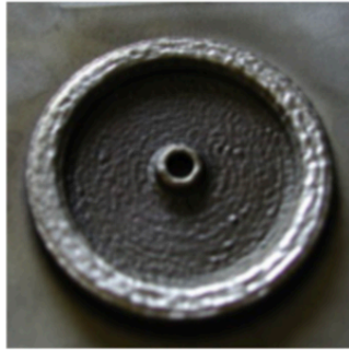
Fig. 32. Functionally graded flywheel (outer radius 0.2 m) composed of 320 stainless steel and copper coated nickel produced using the LENS process [233].
