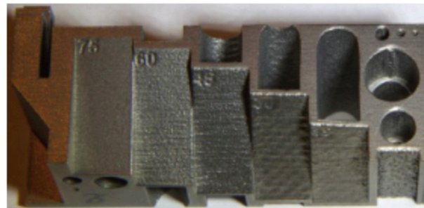
Fig. 38. Benchmark showing the surface roughness resulting for SLM parts with different build angles. Courtesy of ASML.
