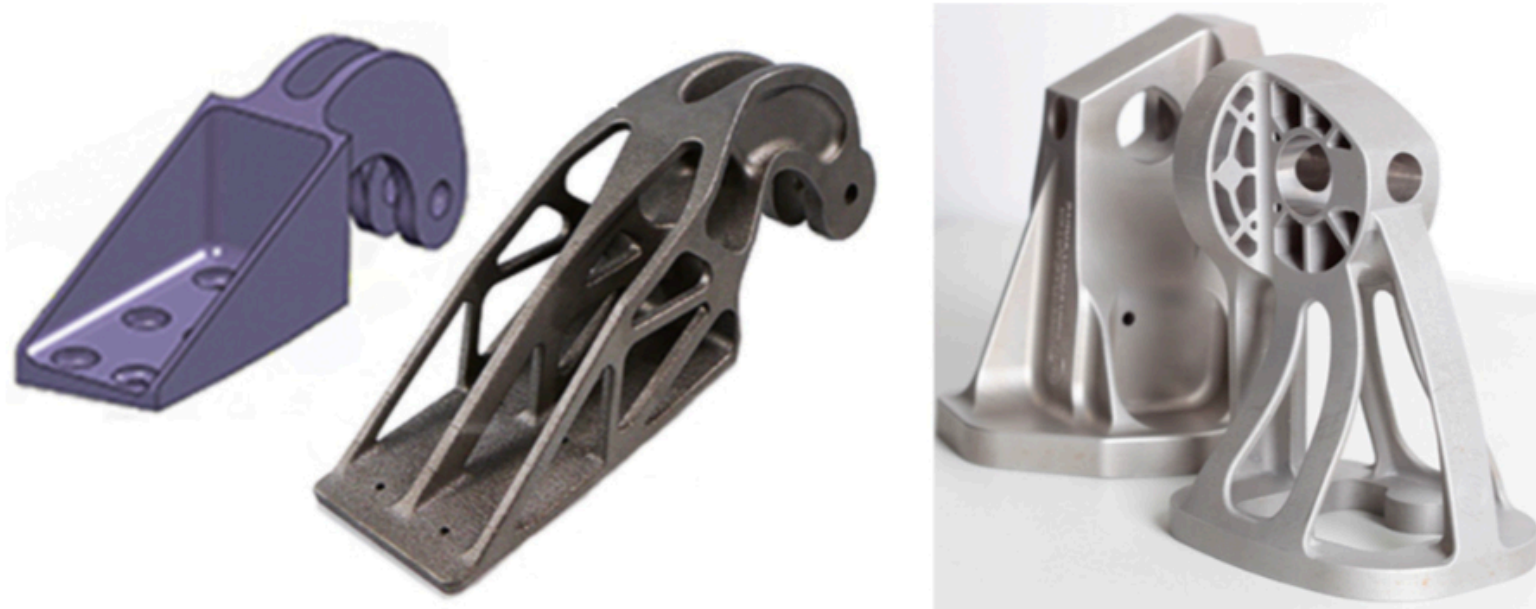
Fig. 16. Brackets before and after topology optimization: Airbus A320 nacelle hinge brackets as-designed for cast steel and optimized for titanium (left) and Airbus A380 brackets as designed and optimized for stainless steel (right) [105]. The optimized brackets were produced by direct metal laser sintering (DMLS).
