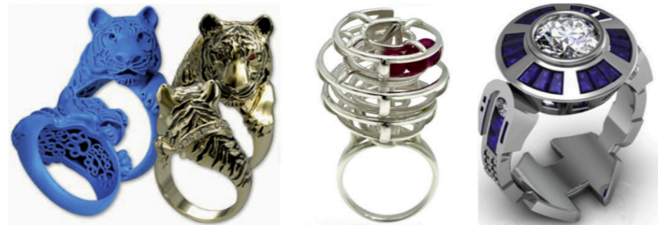
Fig. 9. Jewelry produced with AM: award winning Tiger Ring from OG-Art – pattern printed in wax on a Solidscape machine (via [34]) (left); Kinetic Ring from Vulcan Jewelry (available for purchase) (center, courtesy of Vulcan Jewelry); custom R2D2 inspired ring from Uptown Diamond and Jewelry – pattern printed in wax on a 3D Systems ProJet machine [4] (right).
