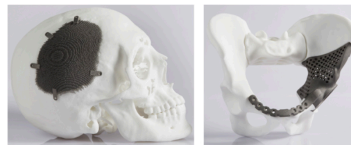
Fig. 18. Titanium implants for the skull (left, [103]) and pelvis (right, [107]) produced using an EOSINT M 280.
