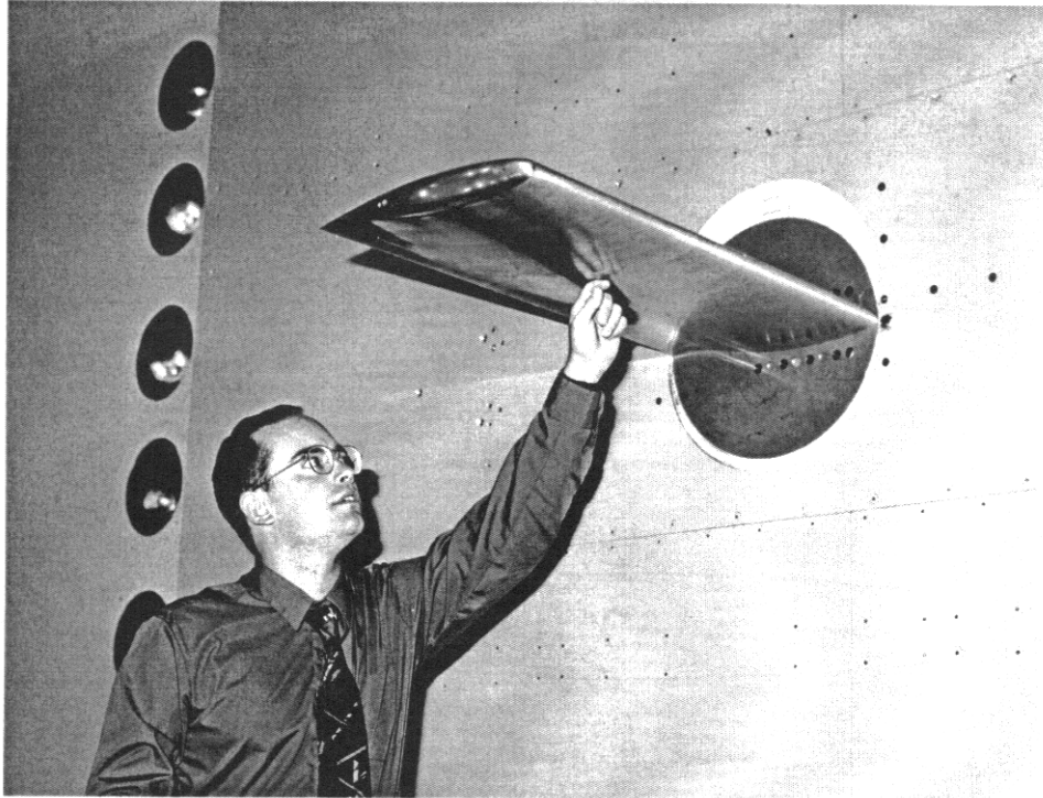
Figure 3. Photograph of Benchmark Supercritical Wing Model mounted in the wind tunnel.
