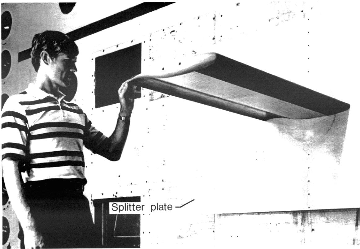
Figure 1. Rectangular supercritical wing installed in wind tunnel.
