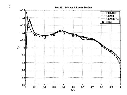
Figure 2 Comparison of EUL3DU and UEMB at section 8 for run 152. Cp is plotted for a) upper surface, and b) lower surface. This figure shows that different tip modelling has less effect than other factors (such as inclusion of viscosity, designated UEMB+vis)
