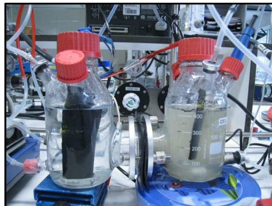
Figure 1: Experimental setup used for the evaluation of dissolved \text{CO}_2 concentration influence on biocathodic reduction for acetate production
