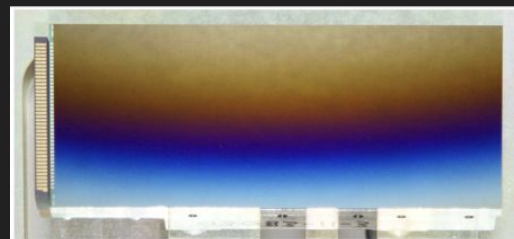
Fig. 14. Picture of the graded-AR coated CCD. The red-sensitive part at the top of the chip looks blue because red light is absorbed while blue light is reflected.
