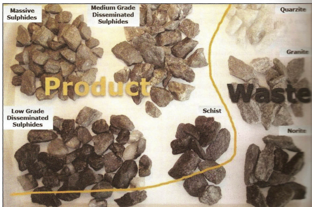
Figure 6. Illustration of XRT sorting—Sudbury nickel ore
