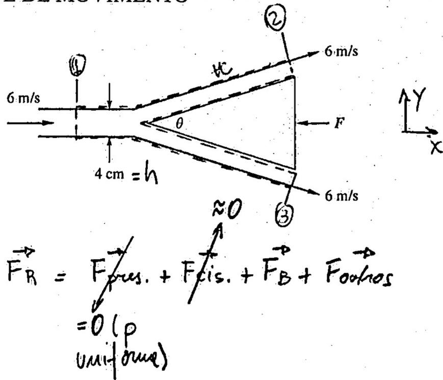
$$\vec{F}_R = \frac{\partial}{\partial t} \int_{VC} \vec{V} \cdot \rho \cdot dV + \int_{SC} \vec{V} \cdot \rho \cdot \vec{V} \cdot d\vec{A} ; \vec{F}_R = F_{pres.} + F_{vis.} + \vec{F}_B + F_{outros}$$
