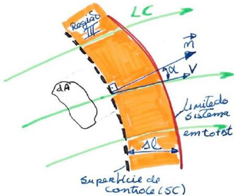
$$\text{termo } B = \lim_{\Delta t \rightarrow 0} \frac{N_{III}|_{t_0 + \Delta t}}{\Delta t}$$
