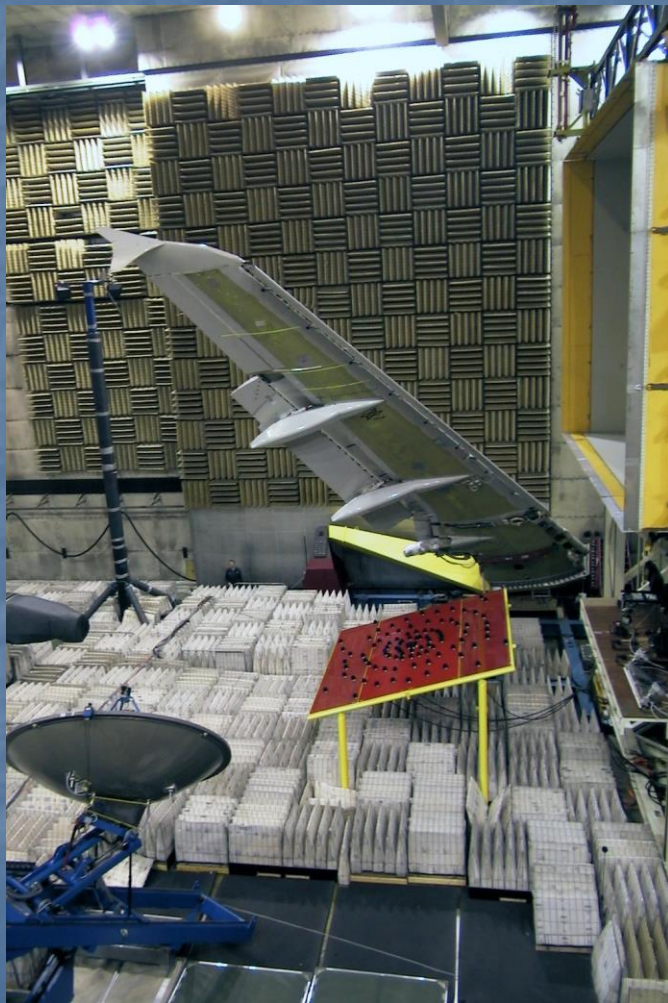
a) A321 with slatless leading edge (landing configuration)
