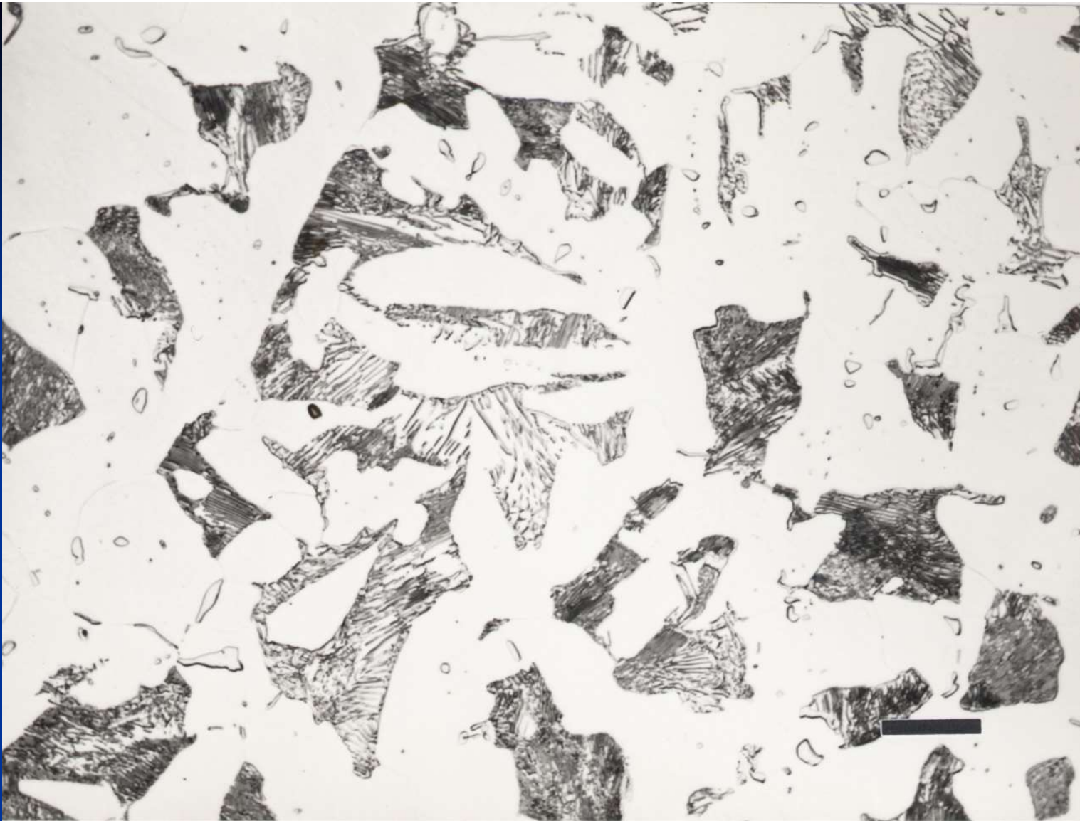
Ferrite (white) and pearlite in a hot-rolled Fe – 0.4% C binary alloy. Picral etch. Magnification bar is 20 \mu\text{m} in length.
