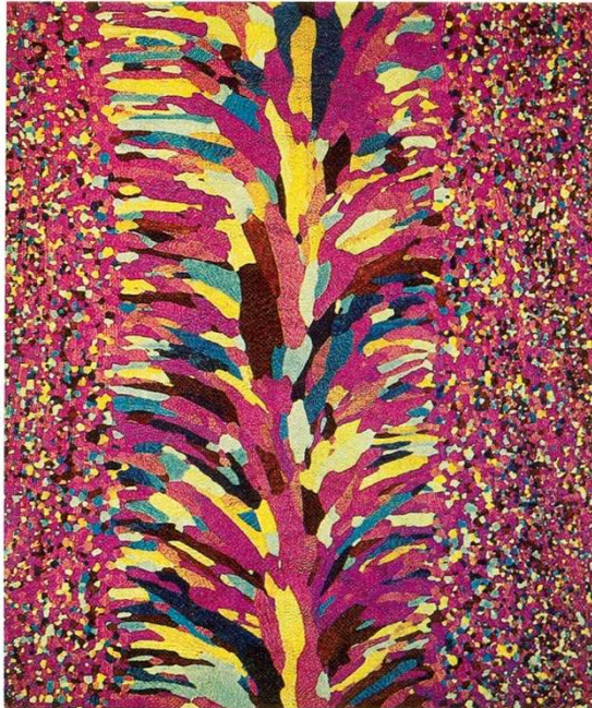
Fig. 32 Electron beam welded 32-mm (1 \frac{1}{4} -in.) thick C103 plate. The vivid grain color separation is due to heat tinting. See Fig. 31 for specimen preparation. 10 \times . (P.E. Danielson)
