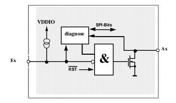
The transmit-function has to be enabled via SPI soft reset after an active RST (low). The open-drain outputs are current-limited, in addition the output voltage on Ax (x=1; 2) is monitored for plausibility. If the voltage at Ax still exceeds a certain defined threshold after switch on the output transistor and after a predefined time tvoff, a short- circuit to battery is detected and the stage is turned off.
