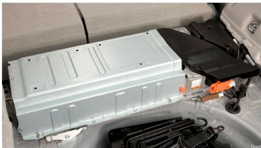
Figura 5.1.4 - HV Battery Pack montado no Toyota Prius 3rd Generation
