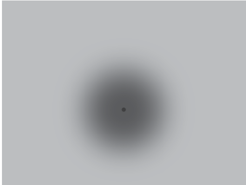
Figure 10.10. The time-average distribution in the normal hydrogen atom. Shading represents density of electronic (negative) charge.
