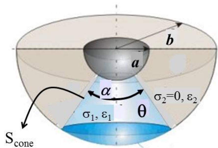
$$\frac{\partial \varphi}{\partial n} \Big|_{S_{cone}} = \frac{1}{r} \frac{\partial \varphi(r)}{\partial \theta} \Big|_{\theta=\alpha/2} = 0$$
