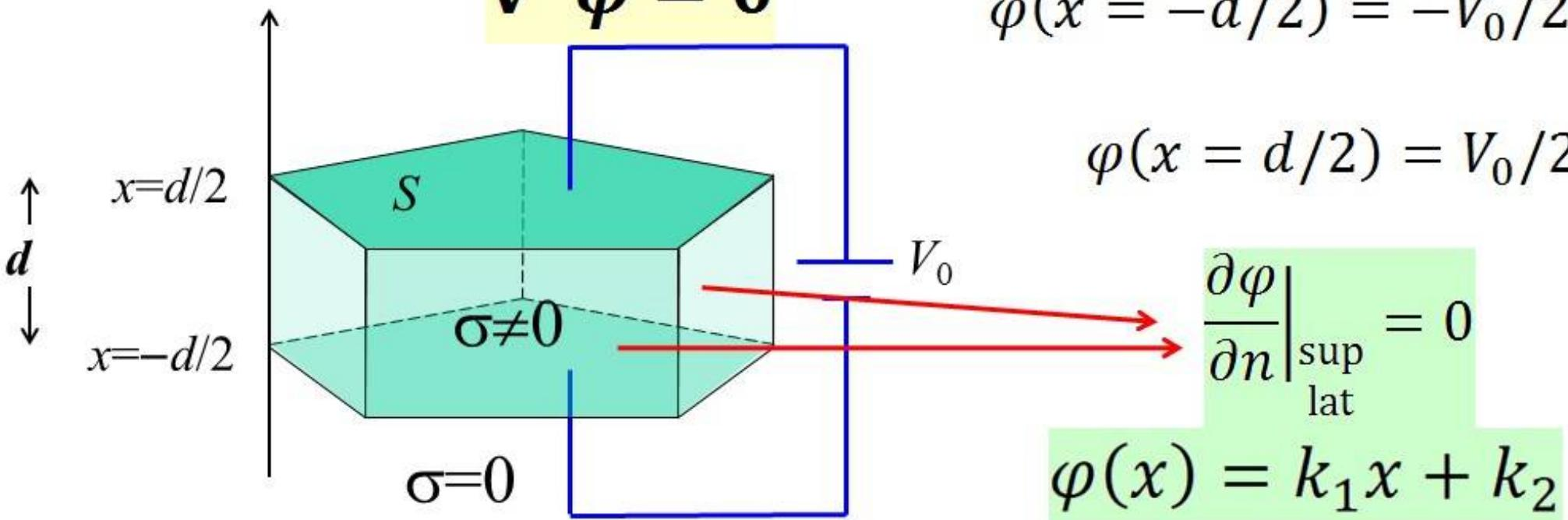
$$-k_1 d/2 + k_2 = -V_0/2 \quad \rightarrow \quad k_1 d/2 + k_2 = V_0/2$$
