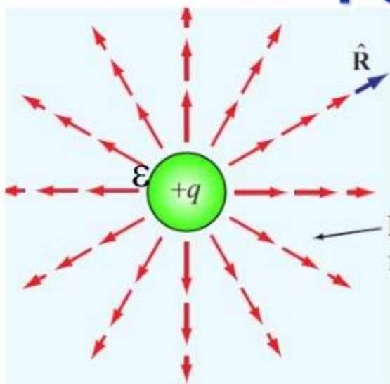
$$\nabla^2 \varphi = 0 \rightarrow \frac{1}{r^2} \frac{\partial}{\partial r} \left( r^2 \frac{\partial \varphi}{\partial r} \right) = 0$$
