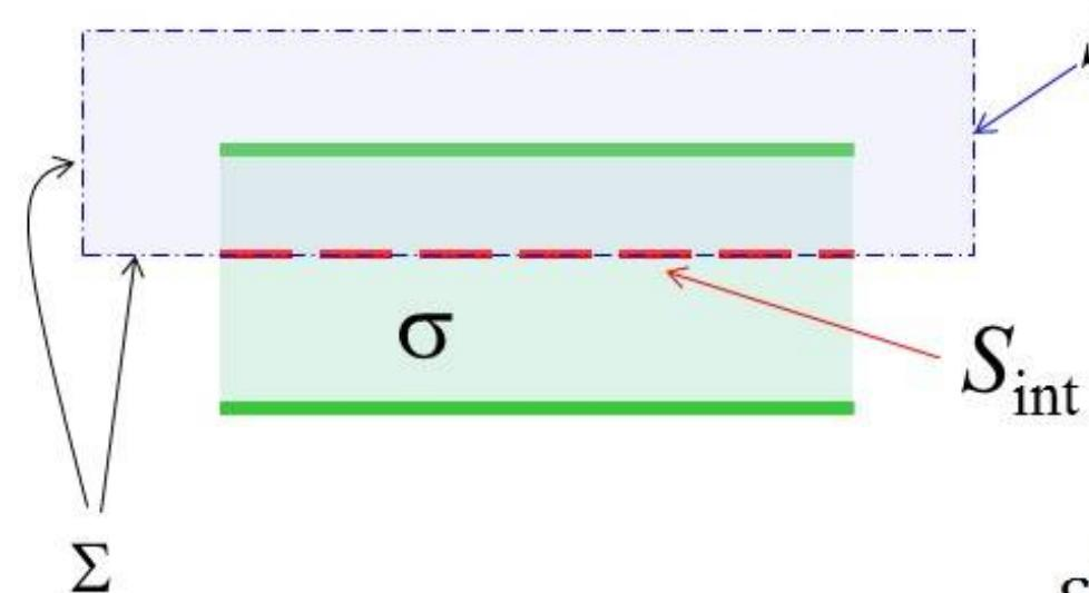
$$S_{\text{ext}} = \frac{\varepsilon V_0 S}{d} + \iint_{S_{\text{ext}}} \vec{D} \cdot d\vec{S}$$
