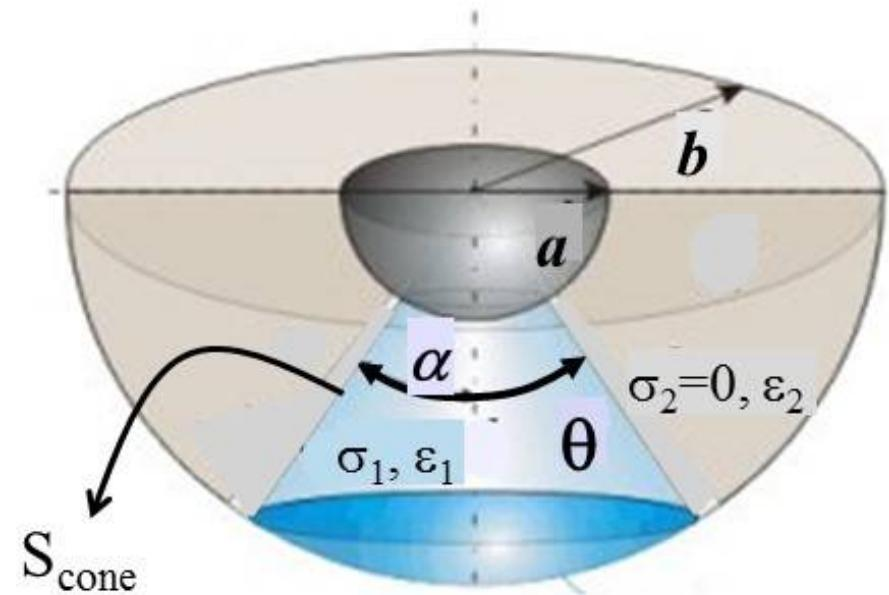
$$\varphi(r) = \frac{V_0}{\left(\frac{1}{a} - \frac{1}{b}\right)} \left( \frac{1}{r} - \frac{1}{b} \right)$$
