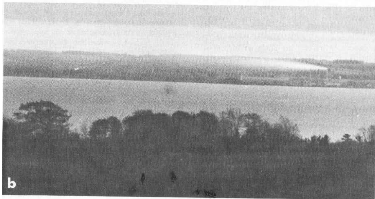
Fig. 3.8 — Plume photographs. (a) Instantaneous ( 1/50 -sec) exposure photograph of a plume. (b) Time exposure (5-min) of same plume. (From Culkowski, 1961.)
