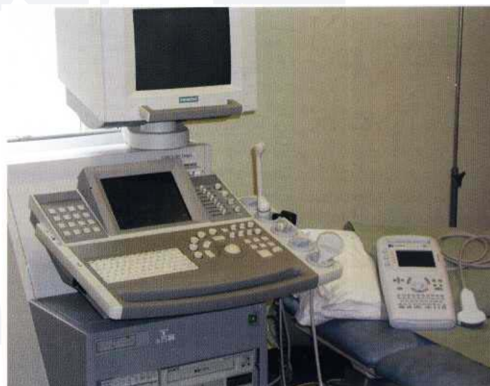
Fig. 59.23 Two modern ultrasound systems, the larger one on the left is a fully configured system; the smaller one on the right on the couch is nevertheless capable of abdominal and small parts examinations, including Doppler studies.
