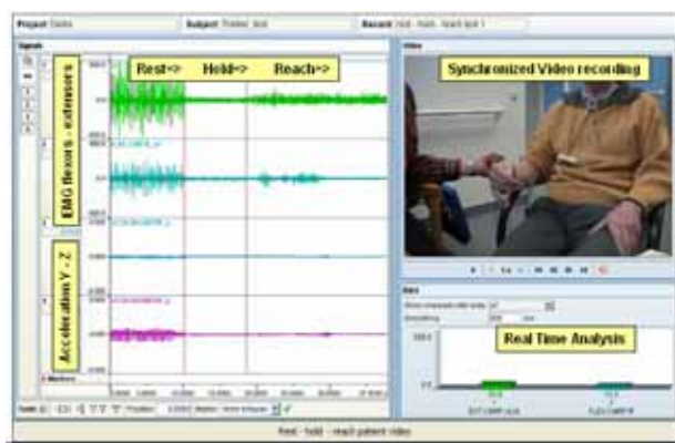
Fig. 1: Combined recording of 2D accelerometer (lower two traces) and 2 EMG traces (upper traces) with synchronized DV-video
