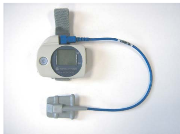
Figure 2.2 An example of a finger probe used in home oximetry.
