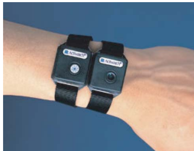
Figure 2.5 An example of a typical actigraph. The person is wearing two varieties of a commonly used device.
