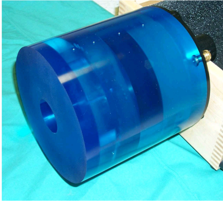
Figure 2. The computed tomography (CT) phantom. This phantom has several regions to test image quality such as low contrast detectability and spatial resolution.
