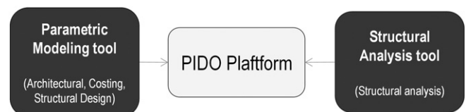
Fig. 3. Tool integration in a PIDO platform to simulate a design process.
