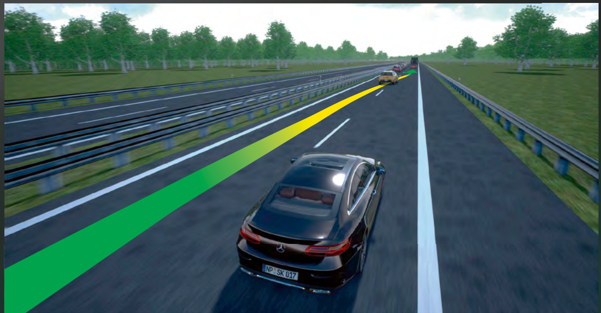
Non-critical cut in because of low value of deceleration, high distance between system vehicle and object.
