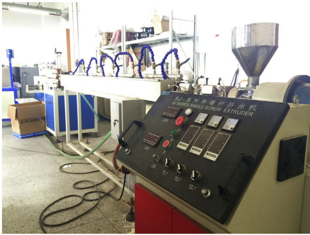
Fig. 3. General view of single screw extruder used in the production of the ABS/OMMT nanocomposites filament.
