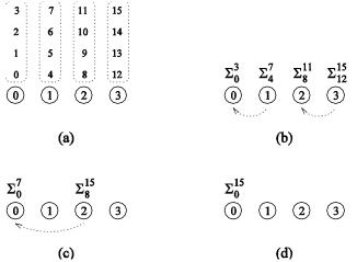
A cost-optimal way of computing the sum of 16 numbers using four processing elements.
