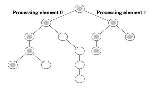
Searching an unstructured tree for a node with a given label, 'S', on two processing elements using depth-first traversal. The twoprocessor version with processor 0 searching the left sub-tree and processor 1 searching the right sub-tree expands only the shaded nodes before the solution is found. The corresponding serial formulation expands the entire tree. It is clear that the serial algorithm does more work than the parallel algorithm.
