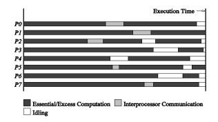
The execution profile of a hypothetical parallel program executing on eight processing elements. Profile indicates times spent performing computation (both essential and excess), communication, and idling.
