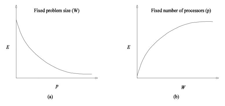
Variation of efficiency: (a) as the number of processing elements is increased for a given problem size; and (b) as the problem size is increased for a given number of processing elements. The phenomenon illustrated in graph (b) is not common to all parallel systems.
