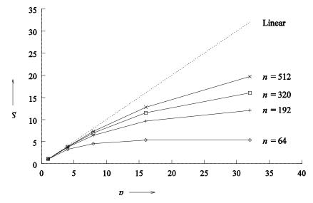
Speedup versus the number of processing elements for adding a list of numbers.
