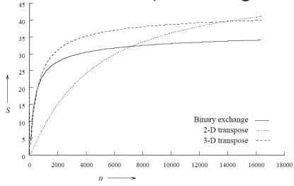
A comparison of the speedups obtained by the binary-exchange, 2-D transpose and 3-D transpose algorithms on 64 processing elements with  $t_c = 2$ ,  $t_w = 4$ ,  $t_s = 25$ , and  $t_h = 2$ .
