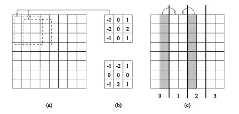
Example of edge detection: (a) an  $\mathbf{8} \times \mathbf{8}$  image; (b) typical templates for detecting edges; and (c) partitioning of the image across four processors with shaded regions indicating image data that must be communicated from neighboring processors to processor 1.
