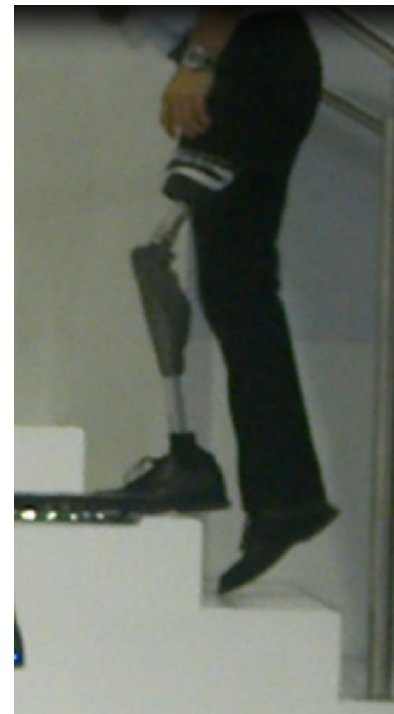
Fig. 18. The Genium® knee (Ottobock) combines a gyroscope and microprocessors to allow the wearer to climb up stairs.
