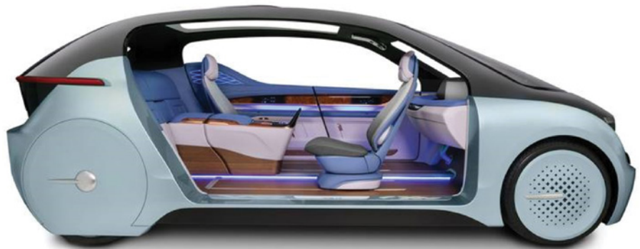
Shuttle-service ACES body with steel-ring easy-access side design and slide-together steel-frame doors can meet side-impact requirements.
