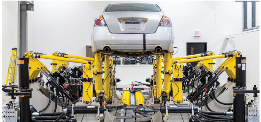
Roush simulator 6DOF: The showpiece of the Roush Advanced Durability Lab is the MTS Systems six-degrees-of-freedom spindle-coupled road simulator.
