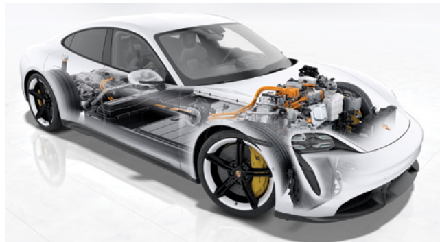
Both variants of the Taycan use a drive motor at each axle and sandwich the lithium-ion battery pack, per current EV norm, in the bodyshell's floor.
