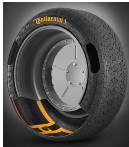
ContiSense incorporates electrically conductive rubber compounds.
