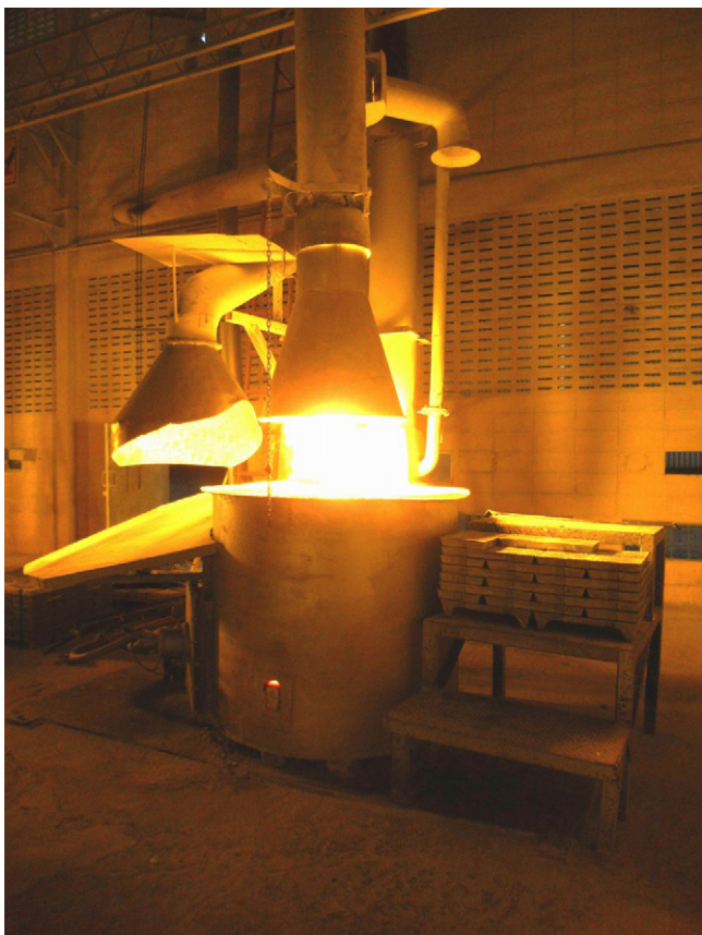
Fig. 4. Photograph of a French process drum in operation, by permission from PT. Indo Lysaght, Indonesia.
