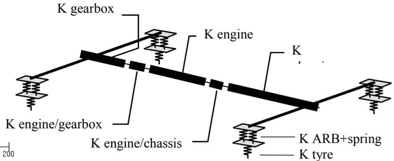
Fig. 4 - Single-seater vehicle model
