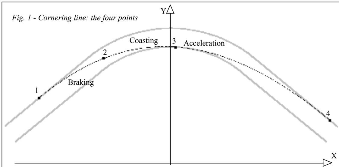
Fig. 1 - Cornering line: the four points
