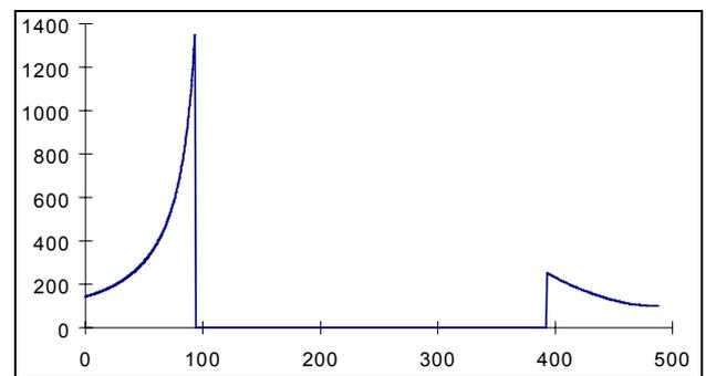
Fig. 5 - Cornering radius along a circuit section
