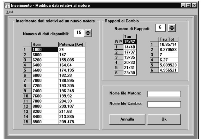
Fig. 13 - Engine power curve and gear ratio input
