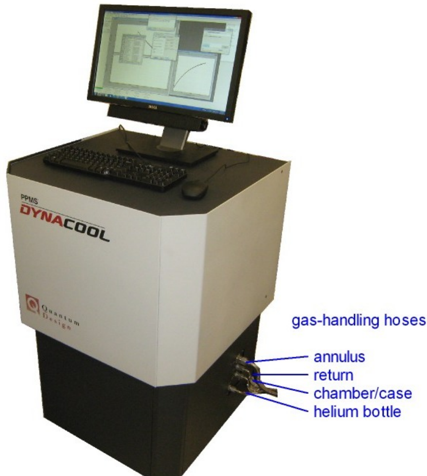
Figure 2-5. Front view of Pump Cabinet.
