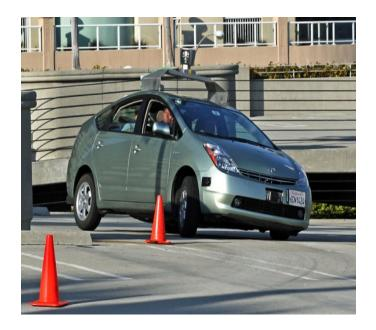
Google's robotic cars have about \$150,000 in equipment including a \$70,000 LIDAR (laser radar) system. The range finder mounted on the top is a <u>Velodyne</u> 64-beam laser. This laser allows the vehicle to generate a detailed 3D map of its environment. The car then takes these generated maps and combines them with high-resolution maps of the world, producing different types of data models that allow it to drive itself.
