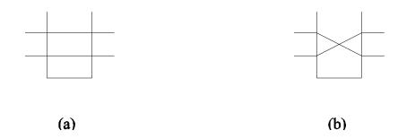
Two switching configurations of the  $2 \times 2$  switch: (a) Pass-through; (b) Cross-over.
