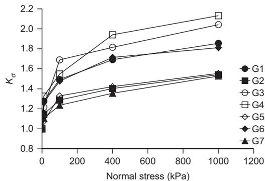
Figure 10. Reduction factor for confinement versus vertical stress
