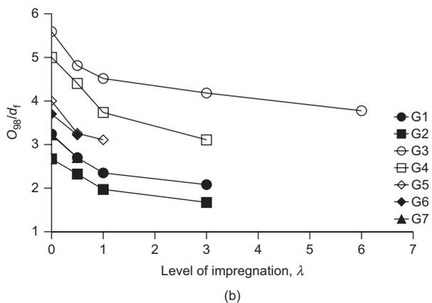
Figure 6. Variation of  $O_{95}/d_f$  and  $O_{98}/d_f$  with geotextile impregnation level – unconfined specimens, (a)  $O_{95}/d_f$  vs.  $\lambda$ ; (b)  $O_{98}/d_f$  vs.  $\lambda$
