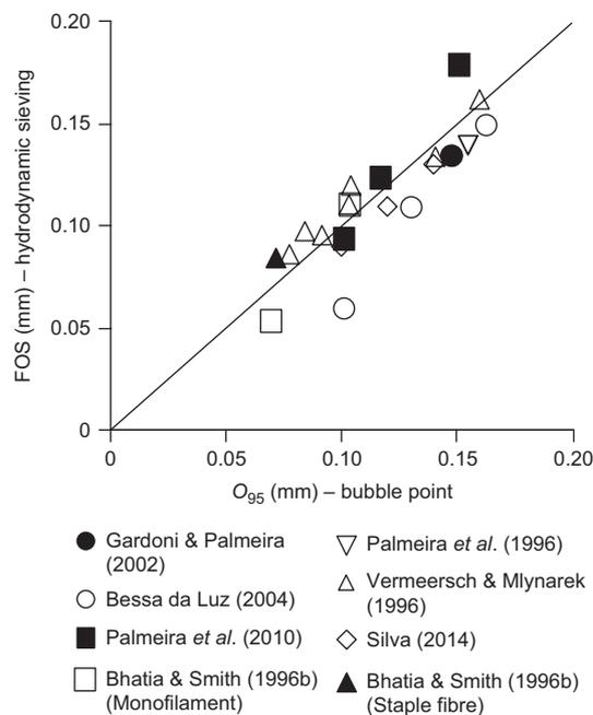
Figure 14. Comparisons between bubble point and hydrodynamic sieving tests – virgin geotextile specimens
