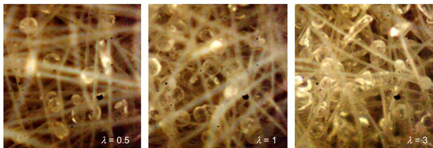
**Figure 3. Images of partially clogged geotextile specimens for  $\lambda$  between 0.5 and 3 (enlarged 200 times)**
