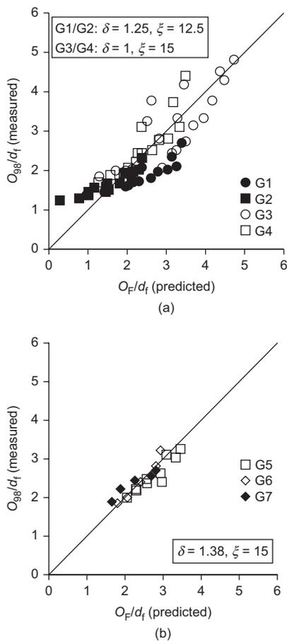
Figure 9. Comparisons between predicted and measured geotextile opening sizes – tests on partially clogged specimens, (a) geotextiles G1 to G4; (b) geotextiles G5 to G7
