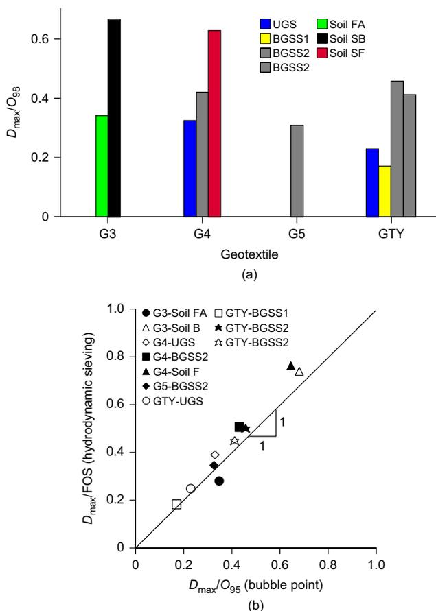
**Figure 15. Ratio between maximum particle diameter and maximum pore diameter after sample preparation in filtration tests, (a)  $D_{max}/O_{98}$  for  $O_{98}$  from BBP tests; (b) bubble point test against hydrodynamic test**
