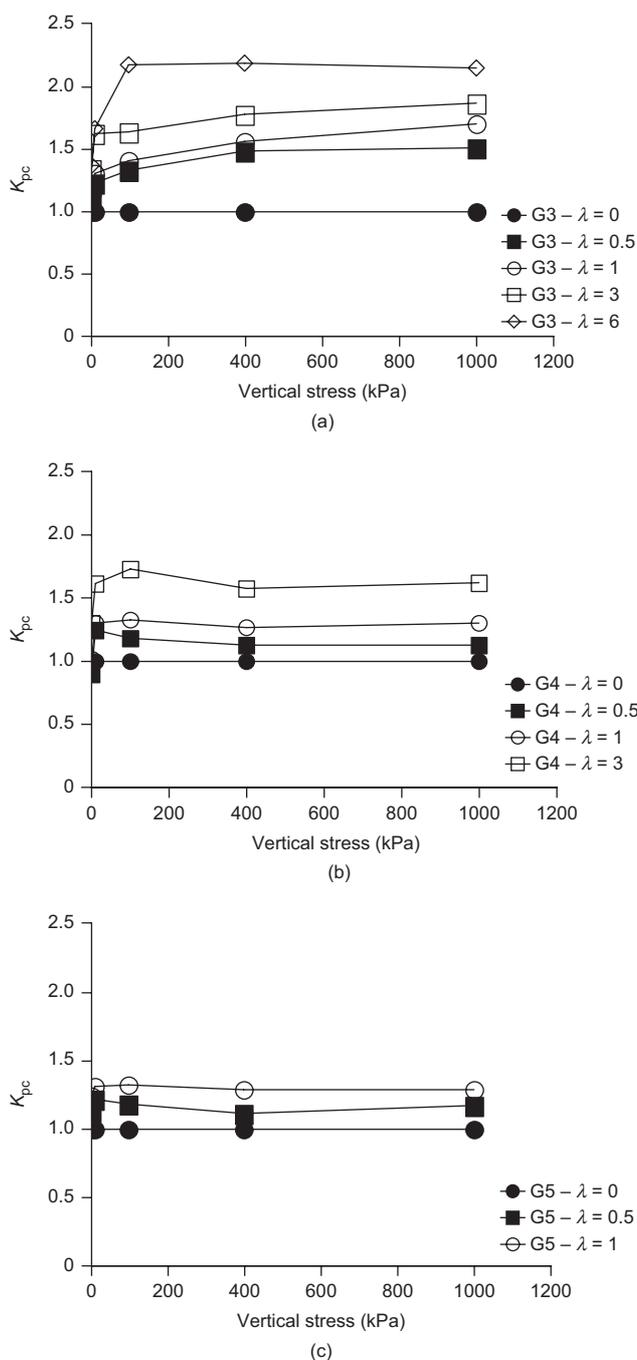
**Figure 12.**  $K_{pc}$  versus geotextile impregnation level, (a) geotextile G3; (b) geotextile G4; (c) geotextile G5
