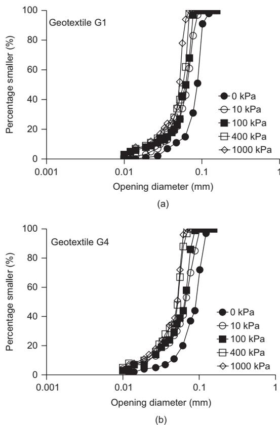
**Figure 4. Pore size distribution curves for geotextiles G1 and G4. (a) G1; (b) G4**
