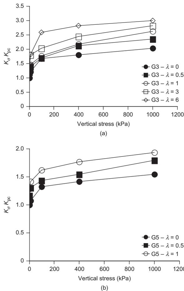
Figure 11.  $K_{\sigma}K_{pc}$  versus vertical stress, (a) geotextile G3; (b) geotextile G5
