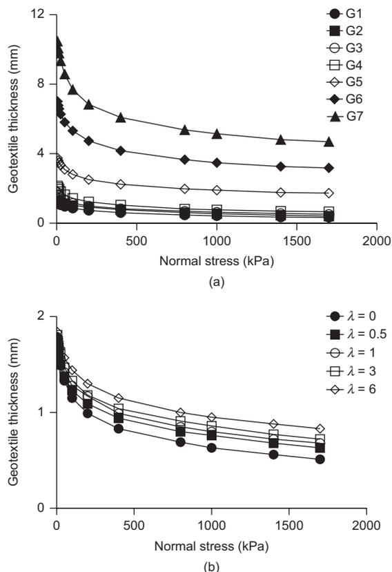
**Figure 2. Results of uniaxial compression tests on virgin and partially clogged geotextile specimens. (a) Virgin geotextiles; (b) Partially clogged – Geotextile G3**
