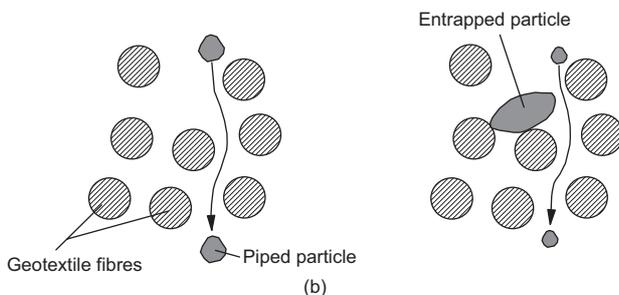
**Figure 16.** Ratio between maximum particle diameter and maximum pore diameter under confinement, (a)  $D_{\max}/O_{95}$  under confinement; (b) reduction of piped particle size due to partial clogging
