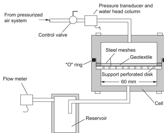
Figure 1. Bubble point test equipment used
