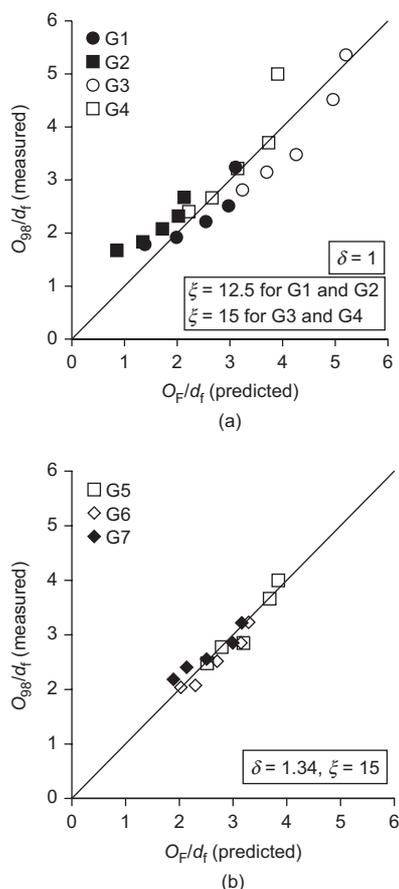
**Figure 8.** Comparisons between predicted and measured geotextile opening sizes – tests on virgin specimens, (a) geotextiles G1 to G4; (b) geotextiles G5 to G7
