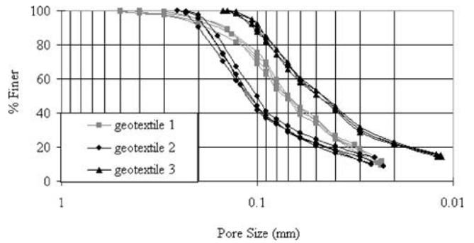
FIG. 4—BPT pore size distributions, showing repeatability.
