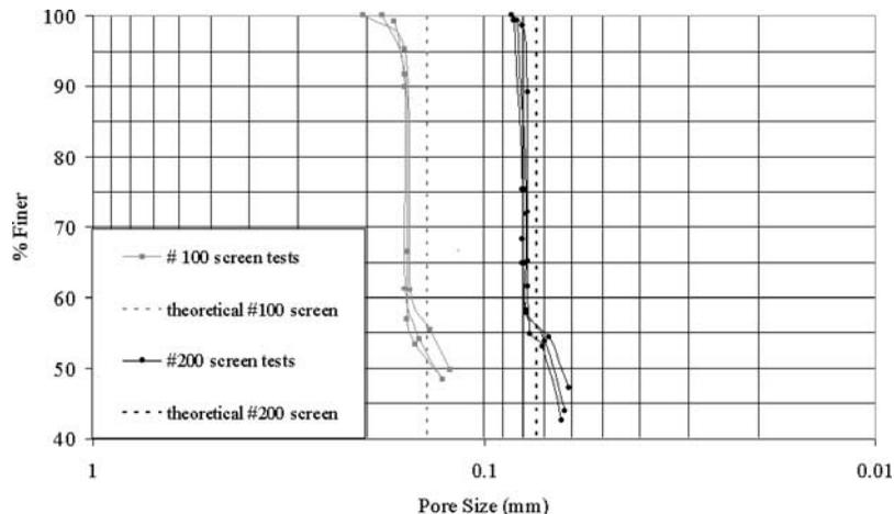
FIG. 5—Pore size distribution from BPT on square hole wire screens.
