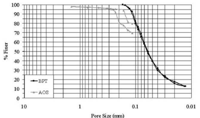
FIG. 8—Pore size distribution: AOS versus BPT for geotextile 5.
