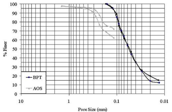
FIG. 7—Pore size distribution: AOS versus BPT for geotextile 4.
