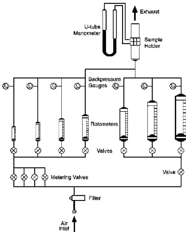
FIG. 1—Schematic of BPT apparatus.
