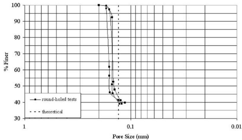
FIG. 6—Pore size distribution from BPT on a round hole screen.
