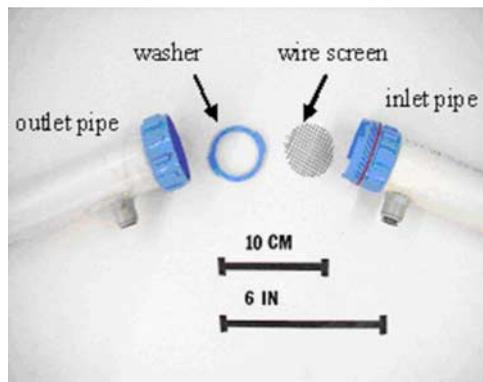
FIG. 3—BPT apparatus sample holder.
