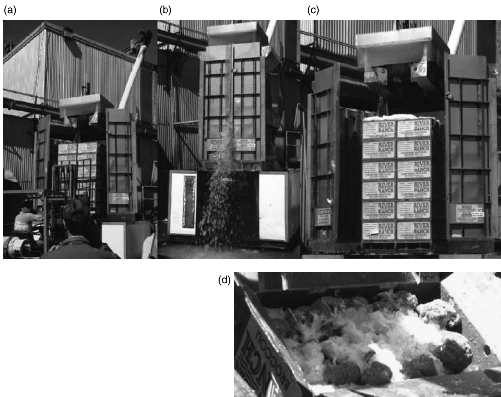
FIGURE 17.33 Liquid ice injecting. Pallets of product that are packed in the field arrive at the cooler and are loaded into the injector (a). A slurry of water and ice is passed through the pallet (b) from top to bottom leaving ice distributed throughout the cartons (c and d).
