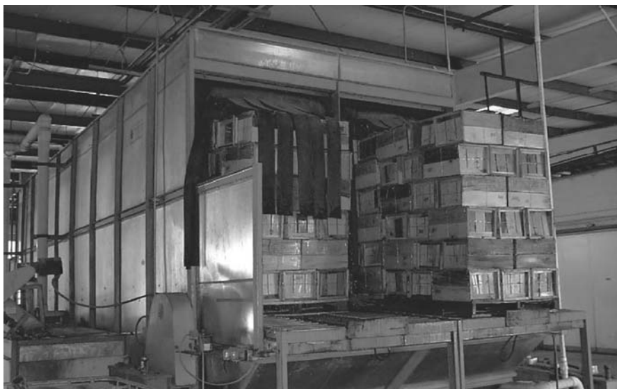
FIGURE 17.32 Conveyer hydrocooling using ice-cold water pumped into a pan over the product that is then showered down through the product.
