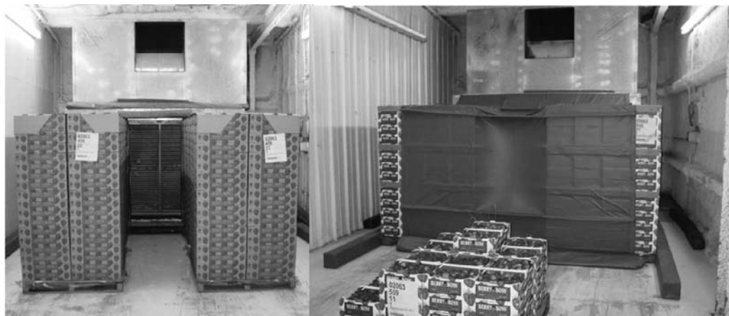
FIGURE 17.31 Tunnel-type forced-air cooling. Two rows of product in ventilated containers are arranged so that an air-return pathway between the rows is left open to the refrigeration coils. A canvas is draped over the product to force air returning to the refrigeration coils to pass through the product. Note air returning under the pallets is blocked by excess canvas in front, and by blocking materials on the sides. Air returns to the room through the opening in the back wall, above the product.
