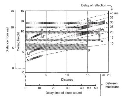
**Fig. 6.12** Influence of hard reflection surfaces on mutual hearing (after Allen, 1980; Barron, 1978; Marshall and Meyer, 1978; and Winkler, 1979). *Angled shading*: favorable reflections; *vertical shading*: unfavorable reflections
