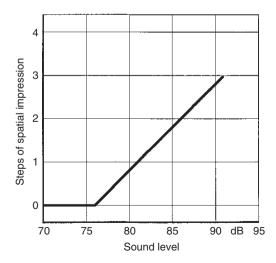
Fig. 5.14 Limiting value of sound levels for onset of spatial impression. Data points for halls (After Kuhl, 1978) from *top* to *bottom*: Stadthalle Hannover, Rheinhalle Düsseldorf, Philharmonie Berlin, Musikhalle Hamburg, Stadthalle Wuppertal. The lowest data point refers to hearing tests with electroacoustic instrumentation
