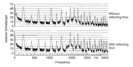
Fig. 7.21 Influence of floor reflections on the tonal spectrum of the clarinet (tone played: A<sub>4</sub>) recorded in anechoic chamber, microphone distance 1.7 m, elevation 1 m
