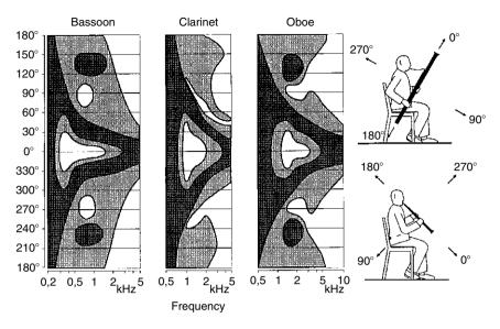
Fig. 4.12 Angular region of principal radiation for oboe, clarinet, and bassoon (average value for entire tonal range)
