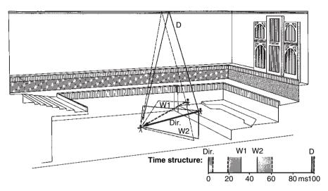
Fig. 8.2 Direct sound and first reflections in a hall originating from the first and last chair of the first violins
