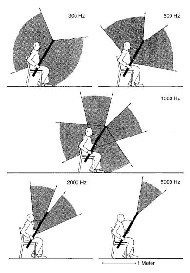
Fig. 7.22 Principal radiation directions (0...-3 dB) for bassoons
