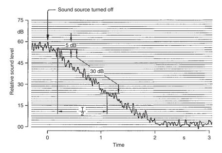
Fig. 5.7 Sound level during a reverberation process
