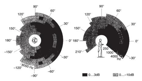
Fig. 4.33 Angular regions of principal radiation regions of the singing voice in octave bands (after Marshall and Meyer, 1985)
