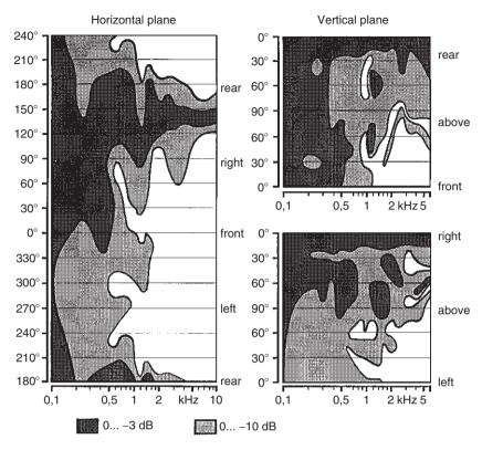
Fig. 4.7 Angular range of the principal radiation regions for the French Horn (with player)
