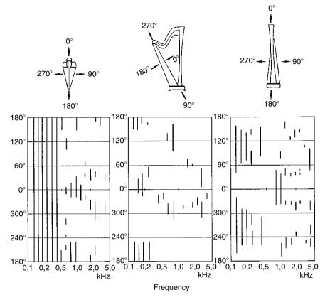
Fig. 4.28 Angular range of principal radiation regions of the harp (0-3 dB after Bell and Firth, 1989)
