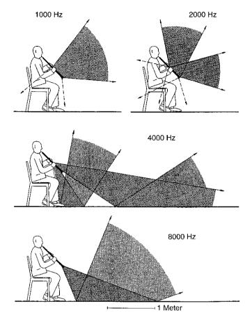
Fig. 7.19 Principal radiation directions (0...-3 dB) for oboes
