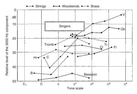
**Fig. 9.6** Relative strength of sound power level of 3,000 Hz components (refer to the strongest partials) for a *forte* sound of solo singing voices and orchestra instruments
