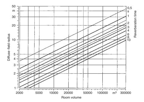
Fig. 5.11 Dependence of diffuse-field distance on room volume and reverberation time (for omnidirectional sound sources)
