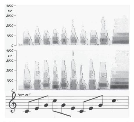
**Fig. 7.28** The sonagram of the *staccato* tone sequence recorded at 3.5 m distance in front of the layer in an anechoic chamber. *Top*: without reflecting rear wall. *Bottom*: with reflecting rear wall
