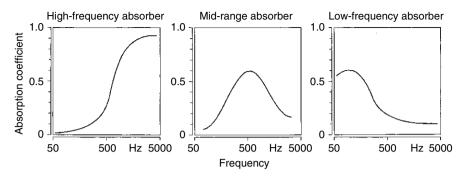
Fig. 5.6 Degree of absorption of materials for differing frequency dependence
