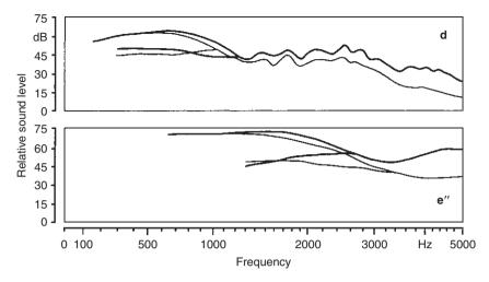
Fig. 8.17 Envelopes of sound spectra of a clarinet for different instrument positions recorded in direction of sight (horizontal) of the player. Thin line: normal position; thick line: bell raised
