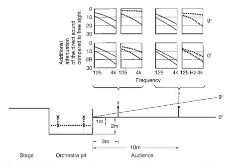
**Fig. 6.18** Shading of the direct sound from the orchestra pit into the audience. In the individual diagrams the *upper curve* relates to musicians close to the stage, the lower ones to musicians close to the audience. *Broken*: orchestra location- high. *Solid*: orchestra location – low
