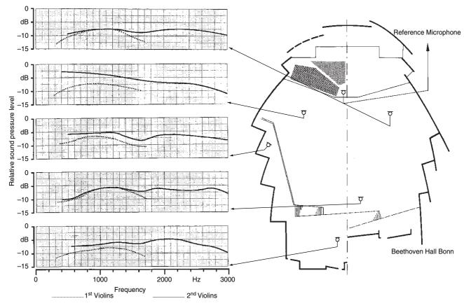
Fig. 7.7 Sound level difference of violins at different locations in the hall compared to the level at the conductor
