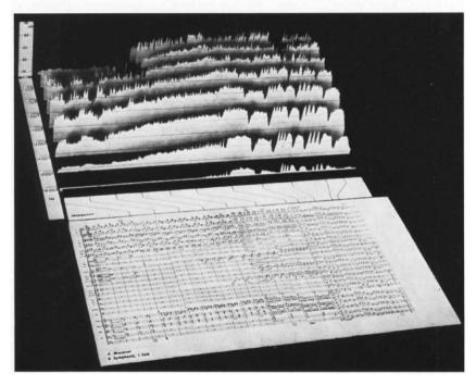
**Fig. 7.31** Octave level models of the orchestral sound in the Stadthalle Braumschweig (A. Buckner, 9th symphony, 1st movement, measure 51–71). *Top*: sound at conductor location. *Bottom*: sound in the 5th row of the main floor
