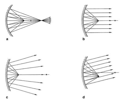
Fig. 5.2 Reflection from curved surfaces
