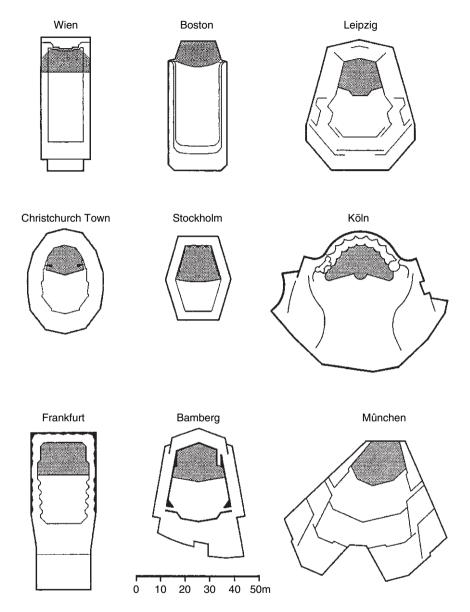
Fig. 6.13 Floor plans of several concert halls. The shaded areas identify the stage
