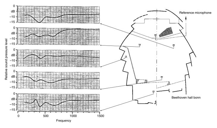
Fig. 7.12 Level differences of Celli at various locations in the hall in comparison to the level at the location of the conductor.
