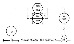
Figure A4. Computer Control-Full Backup from Distribute Control Instrumentation. Computer Uses Instrument System Communication Link
