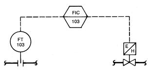
Figure A1. Computer Control-No Backup - Shared Display
