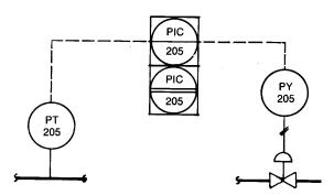
Figure A6. Shared Display/Shared Control—With Auxilia Operator's Interface Device
