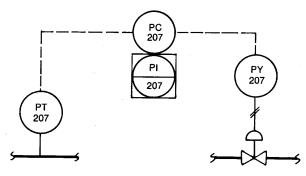
Figure A9. Analog Control-Blind Controller. Shared Display
