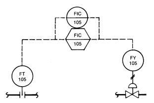
Figure A2. Computer Control-With Analog Backup
