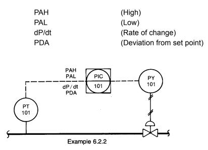
6.2.3 Alarms on controller output shall use the undefined variable identifier X, i.e.:
