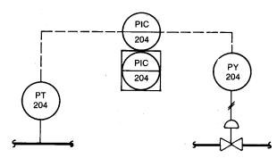
Figure A7. Analog Control—Interfaced with Shared Display. Shared Control Backup
