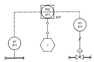
Figure A13. Supervisory Set Point Control—Shared Display Shared Control with Full Computer Access via the Communication Link
