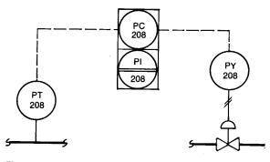
Figure A10. Blind Shared Control—With Auxiliary Operator: Interface Backup
