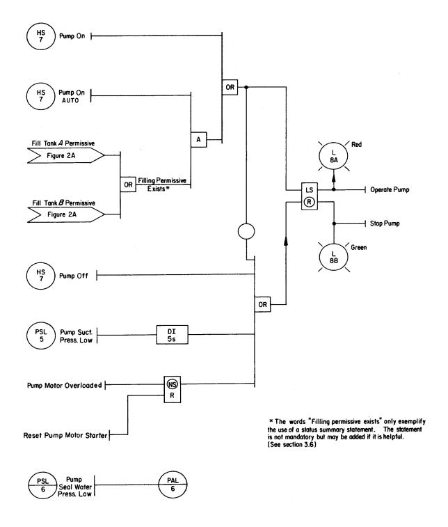
Figure A.2B — Tank filling operation interlock 1 logic diagram — part II
