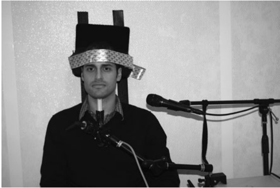
Figure 18.2.3. The head and transducer stabilization set-up at New York University. The ultrasound transducer is restrained with a Magic Arm and the head is held with a moldable head stabilizer.
