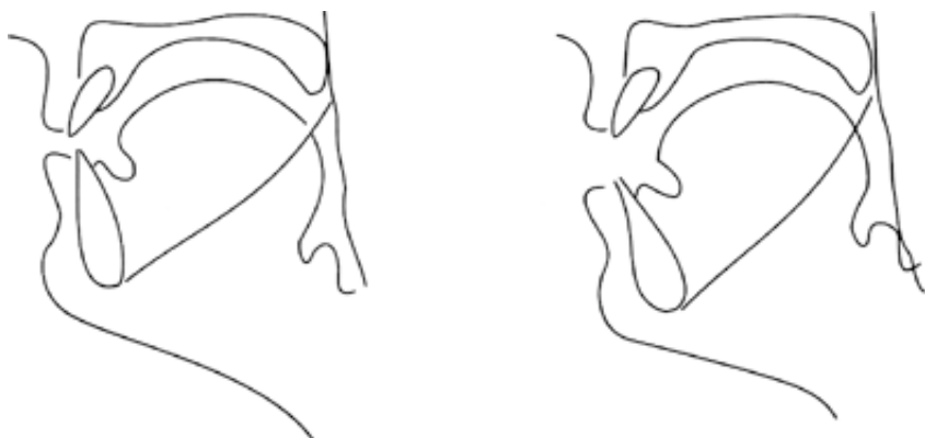
Figure 20.1 Schematic representation of the effect of jaw rotation. A 10° shift in jaw angle moves the lips apart more than the tongue back and velum.
