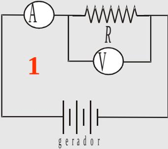
$R_{\text{medido}} = \frac{R_{\text{volt}} R_R}{R_{\text{volt}} + R_R}$ | 1          | 100          | 4.047.519      |
