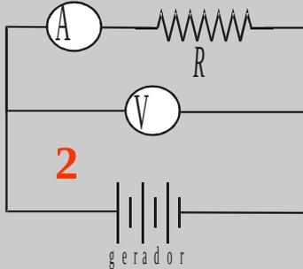
$R_{\text{medido}} = R_{\text{amp}} + R_R$                             | 3          | 102          | 6.800.002      |
