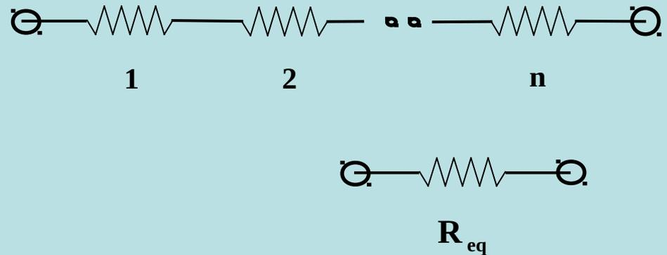
$$R_{eq} = R_1 + R_2 + \dots + R_n$$
