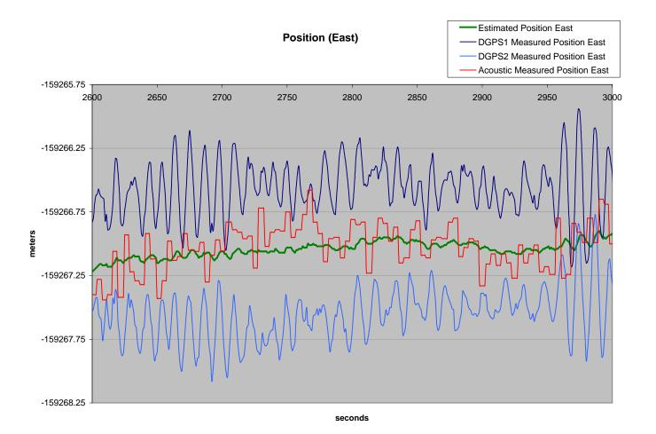
Figure 8 – Example of Estimated Position (East) compared to Position Reference System measurements (after pre-processing) – Deepwater Frontier, Brazil
