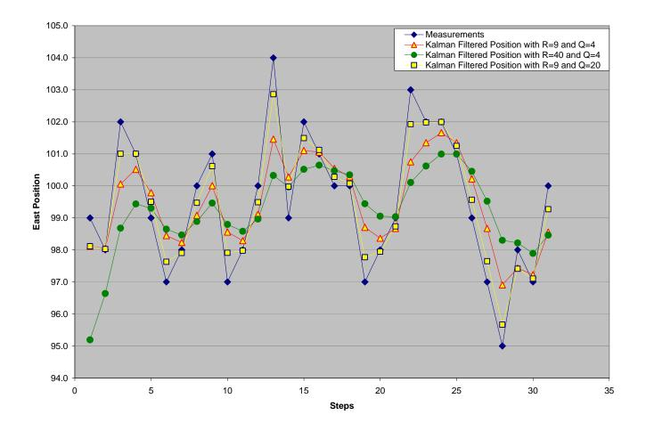
We can also visualize with this example the effect of changes in the Process Noise Covariance Q and the effect of changes in the Measurement Noise Covariance R.
