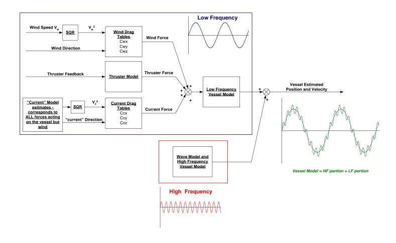
Figure 3 – Block Diagram of Typical Model (simplified)
