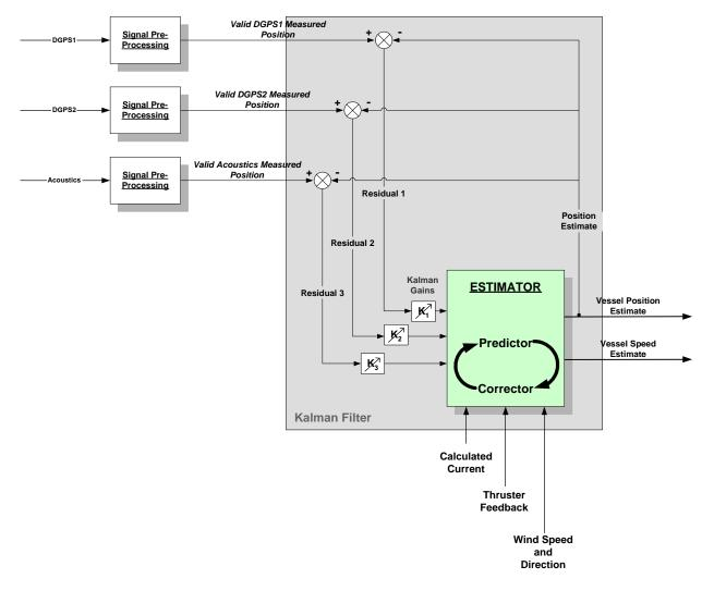
Figure 7 – Simplified schematic of Kalman filter (one possible implementation)
