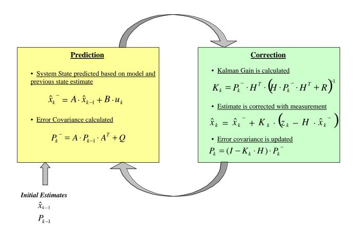
Figure 5 – Predictor-Corrector Structure of Kalman Filter with Equations
