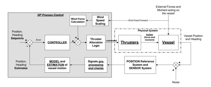
Figure 1 - Functional overview of a Dynamic Positioning control system
