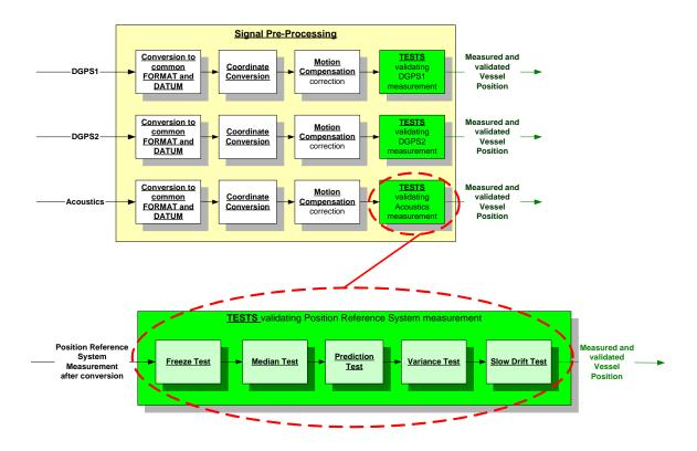
Figure 2 – Typical Position Reference System Pre-Processing Routines
