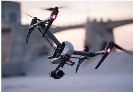
A DJI Inspire 2 flown in Los Angeles. The camera hangs below and the landing gear rises up out of the frame.
