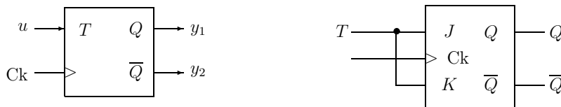
Figure 1.5.16: Edge-triggered T Flip-Flop: Block diagram and construction from an edge-triggered J-K flip-flop
