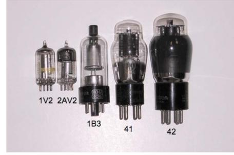
Fig. 1. Representative vacuum tubes used in this study. The 1V2, 2AV2, and the 1B3-GT are vacuum diodes and were used to measure  $e/m$  using the Childs–Langmuir equation (4). The type 41 and type 42 vacuum tubes are power amplifier pentodes. All tube types possess concentric cylindrical geometry.
