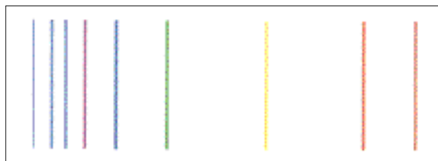
Fig. 1. Nine observed lines of the helium spectrum. In many discharge tubes the yellow and green lines show dimmer lines of the same color right next to them. These “ghost images” are not part of the spectrum and can cause confusion.
