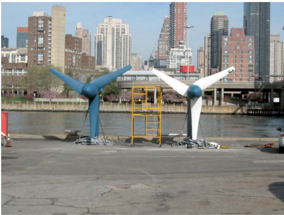
Fig. 1. Two turbines deployed in New York City's East River. The diameter of each turbine is 5 m. (Used with permission of Verdant Power).
